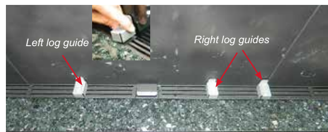
Log guides installed
