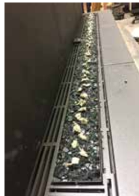
Burner covered with Fireglass and glowing wool
