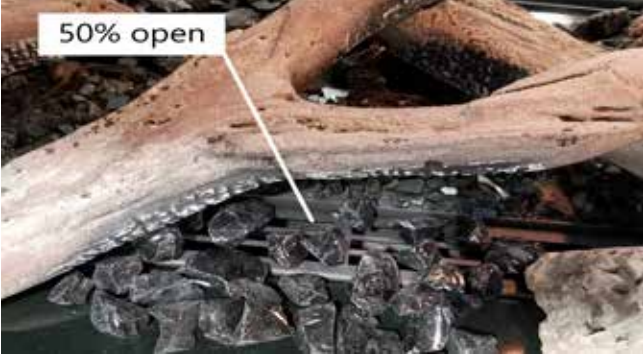
Correct Coal Placement
