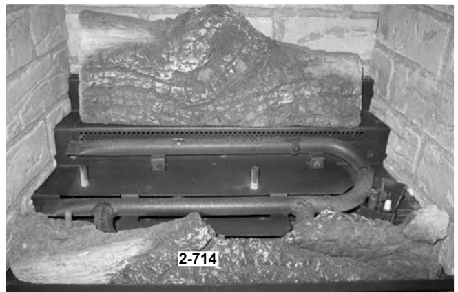
4) Fit log 2-712 into the pins on the middle of the burner.
