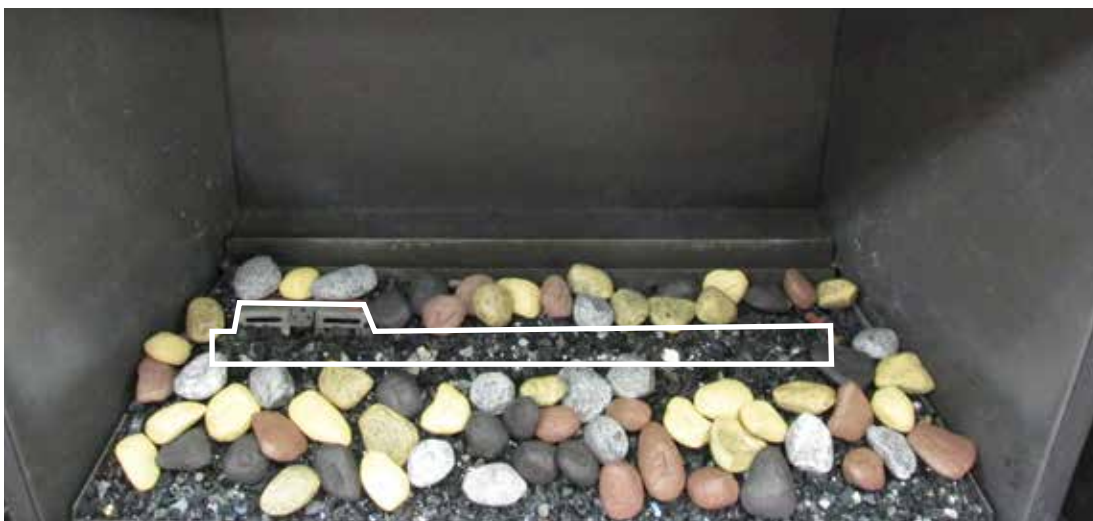
Caution: Do not cover pilot or burner ports with stones.
