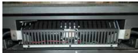
Secure fan with 2 screws removed in Step 1
