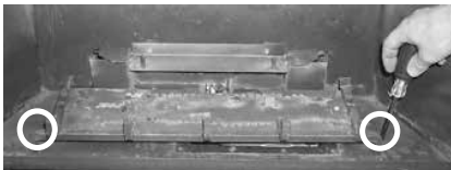
Remove the 2 screws, push Burner Assembly to the left and lift out.
