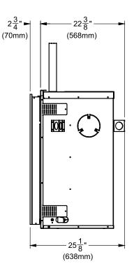
Note: Gas connection is from the right hand side of the appliance & electrical connection on left hand side of the appliance. A metal receptacle box is supplied/installed with the appliance to make all 120 volt electrical connections.
