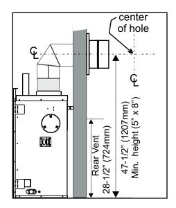
IMPORTANT Must use Rear Venting Deflector packaged with unit in rear vent horizontal termination applications.
