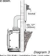
\*As specified in CSA B149.1 Installation Code. Local codes or regulations may require different clearances.
