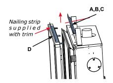
Determine the total thickness of facing material (e.g. drywall or wood plus ceramic tiles) to allow the finished surface to be flush with the front of the unit. Total facing thickness can vary from 1/2" (13mm) to 3-1/8" thick.
