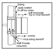
The four wood screws provided should be replaced with appropriate fasteners for stucco, brick, concrete, or other types of sidings.
