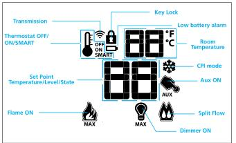
Figure 2: Transmitter LCD Display
