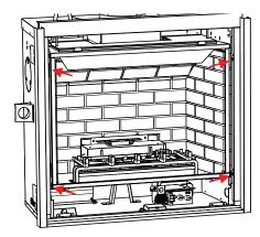
7. Install the lower finishing trim (if required)–secure with four screws.
