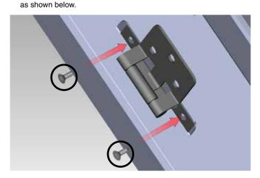
**3.** Flip the hinges down to 90° - line up the lower premium front as shown below.
