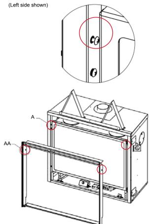
4. Line up Vignette Frame to unit and hook the frame on to the appliance. Slide the top of the frame (See Detail AA above) on to the screws.
