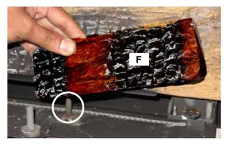
Place Log I on the left side of the burner, directly in front of Log A. Position Log I so it fits into the pin on the burner as shown below.
