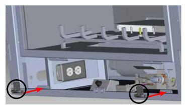
2. Attach the each hinge to the corresponding bracket with 2 screws
