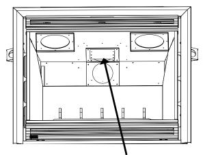
Diagram 2: Vent Restrictor installed on Top Exhaust Assembly
