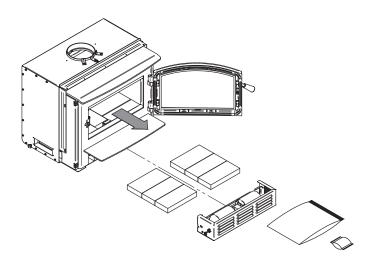
Figure 23: Empty the combustion chamber
