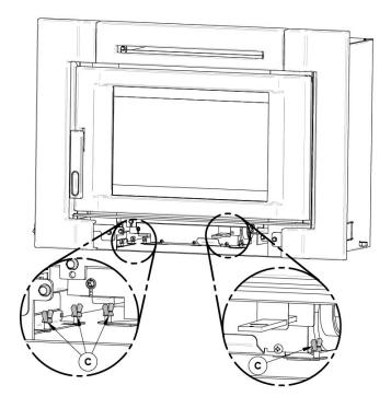
3. Slightly loosen the 4 wings nut (C) then pull the blower assembly (D) towards you to remove it from the convection air jacket. Make sure to disconnect the wiring as it is accessible.
