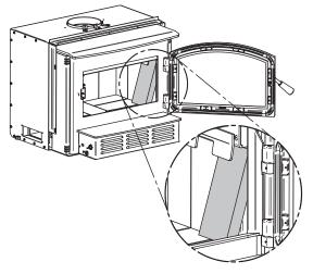
Figure 25: Install the Combustion Chamber Bricks
