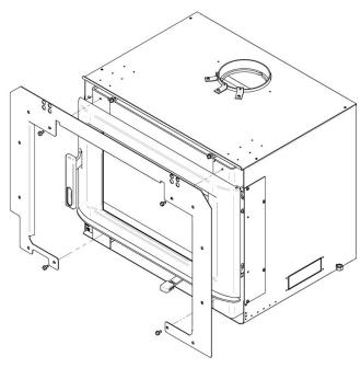
2. Put together the steel face plate with the two parts of the cast iron faceplate.
