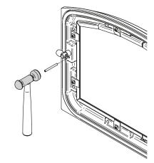
Figure 21: Installing the split pin
