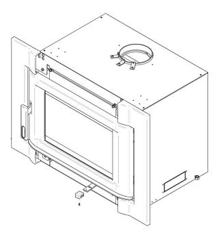
7. Slightly unscrew the two screws at the bottom of the insert. Hook the bottom faceplate and screw it back in place. Reinstall the wood handle.
