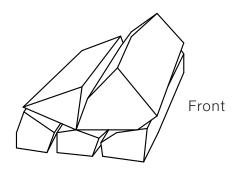
Figure 11: Position of the bottom pieces (High burn)
