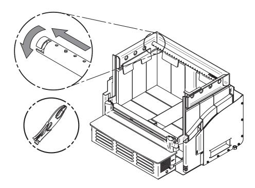
Note that secondary air tubes (A) can be replaced without removing the baffle board (B) and that all tubes are identical.
