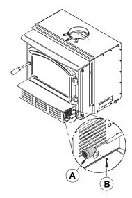
Figure 24: Installing the air control wood handle
