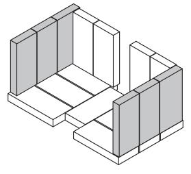
Figure 26: Combustion Chamber Bricks Layout
