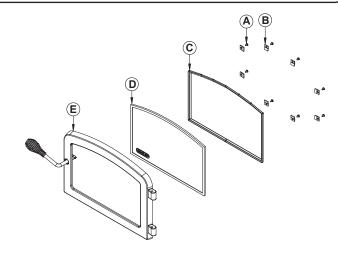
Figure 22: Replacing the glass
