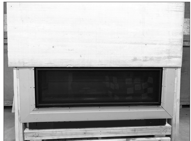
Figure 4.9, Installed Panels and Non-Combustible Material
