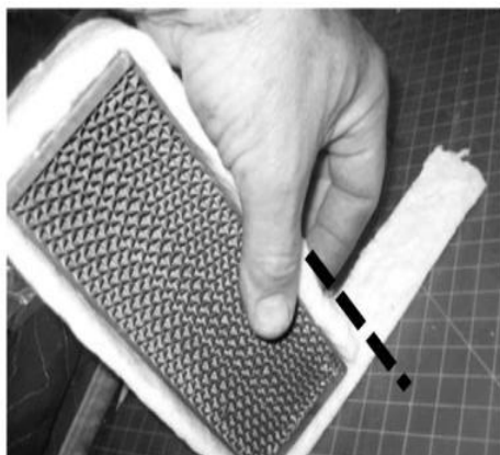
Figure 21 - Installing Gasket on Catalyst
