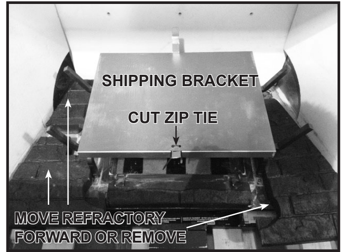
Figure 11.10 Separate Shipping Bracket from Log Grate
