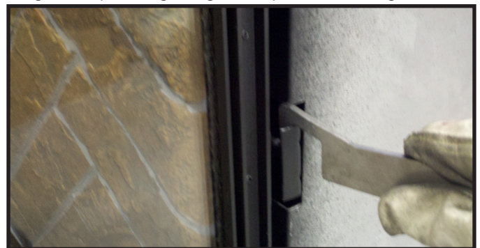
Figure 11.7. Securing Side Glass Clips
