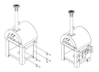
8. Install 3pcs of "L" short hooks and 1pc of long "L" hook with 8pcs of 1/4" \*15mm screws.
