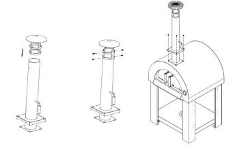
4. Install chimney cap with 4pcs of 5/32"\*10mm screws.
