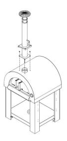
6. Install chimney box with 4pcs of 1/4" 30m screws.
