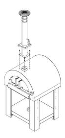
5. Install chimney with 4pcs of 1/4"\*15mm screws.
