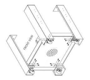
1. Install the bottom shelf with the 16pcs of 1/4" \*15mm screws. Make sure swivel casters w/ brakes are both on the right or left side of the unit.
