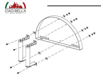
3. Install the door handles with 4 pcs of 1/4"\*15mm screws + insulation mat + flat washer + spring washer + 1/4" bolts. Don't place door on oven until your finish step.
