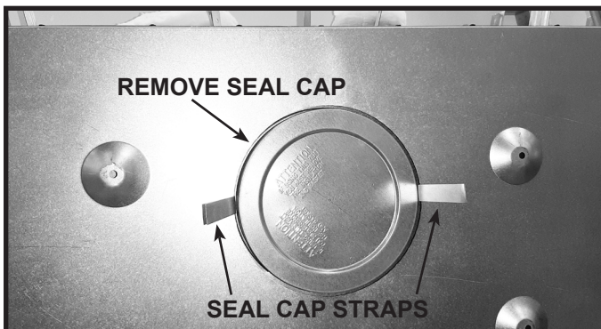
Figure 6.9 Remove Seal Cap
