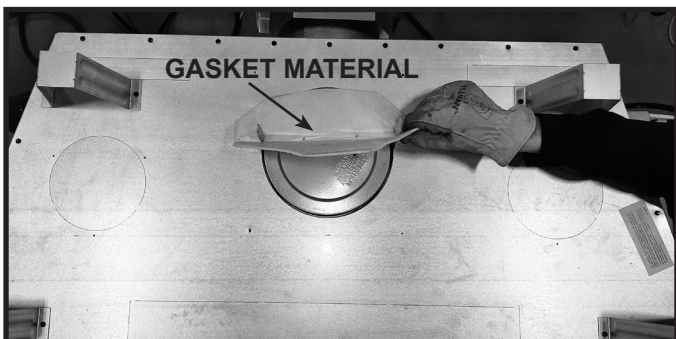
Figure 6.3 Remove the White Gasket Material Covering the Seal Cap
