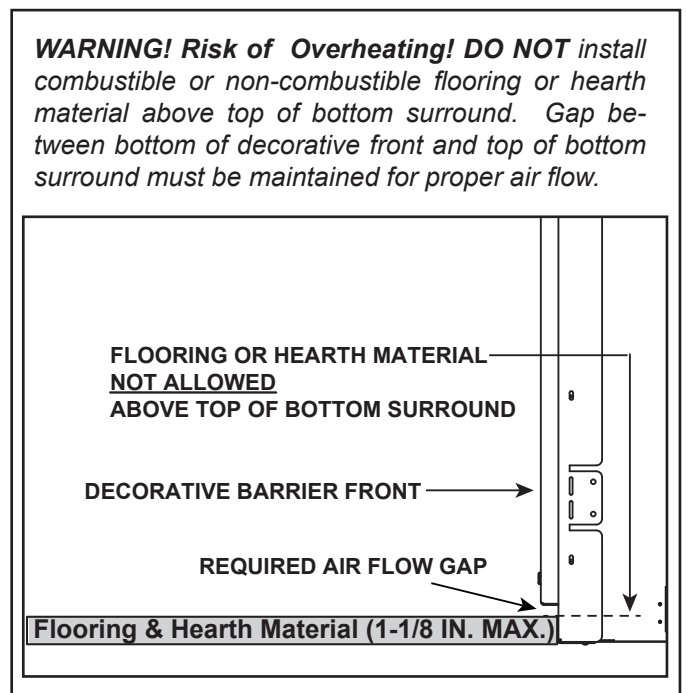
Figure 10.3 Required Air Flow Gap
