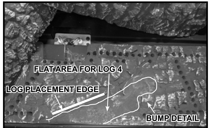
Figure 8 Log Placement Details
